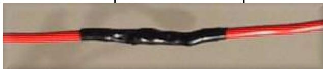
To complete the soldered joint electrical repair, it must be protected from moisture intrusion as well as shorting to a grounded surface. Shrink tubing (of an appropriate size to accommodate the joint) should be applied over the joint while heat is applied. This keeps the joint insulated and waterproof.
