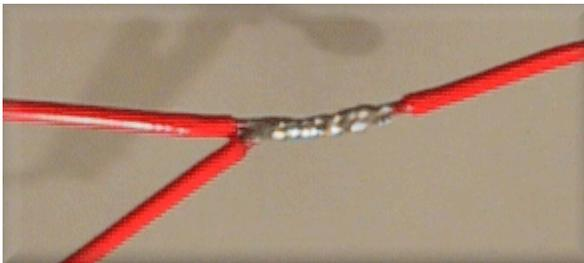
The solder must wet to the surface of the wires its trying to bond to. The greater the surface area that is wet the greater surface area the solder will bond to. In a pair of twisted wires, good surface wetting will result in the solder being pulled into and around the bonding surfaces, maximizing the contact area, providing the most minimal amount of electron interference, keeping resistance to a minimum. This will provide the best possible soldered joint.
