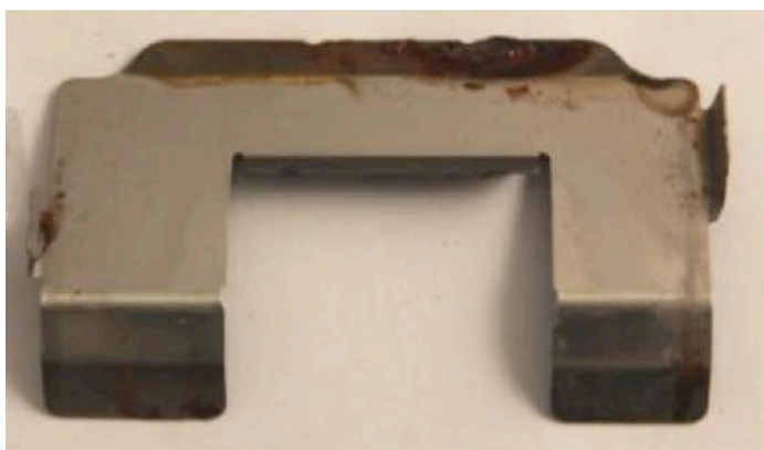
201 Grade Stainless Material After 96 Hour Salt Spray Test Shows Rust and Corrosion
