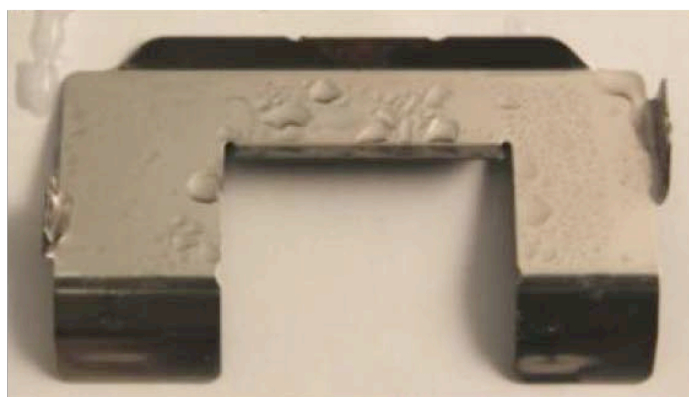
301 Grade Stainless Material After 96 Hour Salt Spray Test No Rusting or Corrosion
